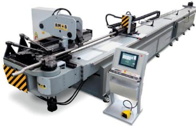
Green's investment in a new CNC multi axis, mandrel and boost bending machine enables production of tube heat exchangers ranging from 25.4mmØ to 114.3mmØ. Green's capability to produce cold formed bends with less than 1D centres whilst increasing efficiency through enhanced automation further demonstrates our commitment to improve productivity and support customers' requirements.
